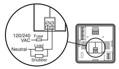
Figure 3.9 Control Output Wiring–R1 and T1
